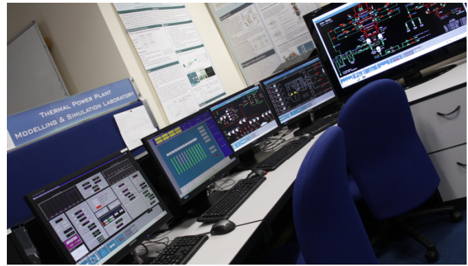
Fig. 3. Several GUI screens from the power plant simulator.
